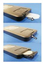
Initial start-up requires the removal of the battery pull-tab.
