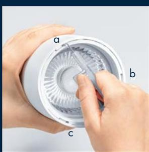
Using the front ring tool (supplied with the lens) push the metal rod into the gap on either side of the plastic pin.
