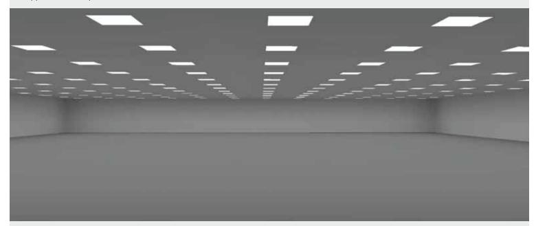
Area: 900m<sup>2</sup> Spacing: 2.4m x 2.4m Polar LED's Wattage: 31W Total Watts: 4,464W (4.96 W/m<sup>2</sup>) Number of Polar LEDs: 144 Average Lux: 376 lux
