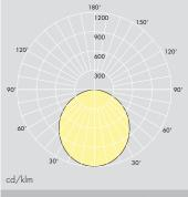
POLAR LED 3000 12X3 4K FP Light source: LEDs 46W C90=C0
