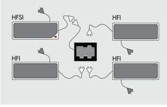
HFI: dimmable with DALI/DSI protocol, HFSI: dimmable with SensaDigital sensor.
