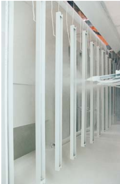
Automatic powder coating paint line using electrostatic application.
