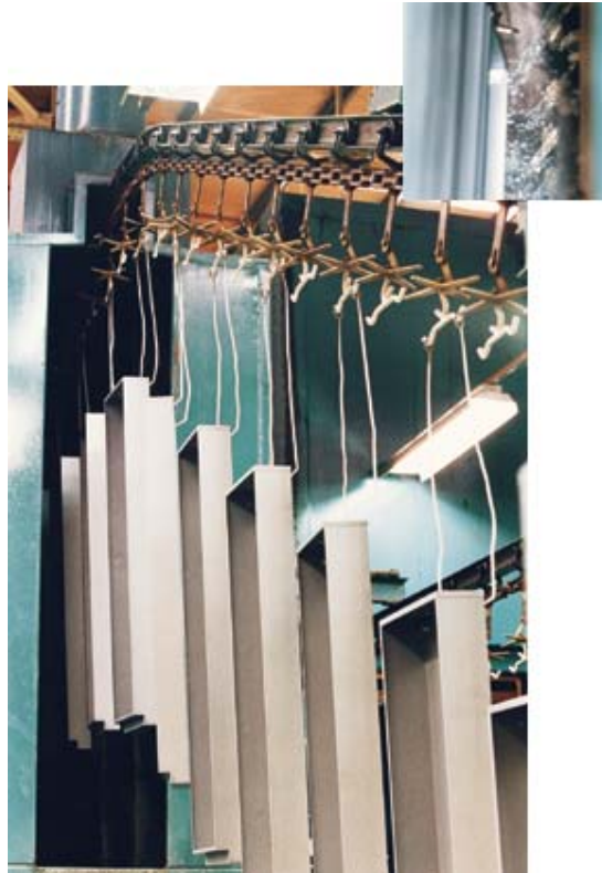
Troffers entering treatment chamber prior to painting. Inset - close up of cold water rinse stage.
