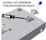
Replace resistor with the alternative item (supplied in plastic bag) and marked with the lower output to be achieved.
