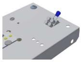
Use a small flat screwdriver and remove the existing resistor.
