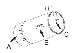
A: Adjust the beam angle via rotating the front ring.
