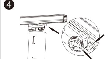
Turn the handle 90 degree to lock the luminarie on the track bar
