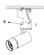
Install the luminarie to the mounting plate by screws
