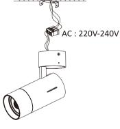
Connect AC cable on the terminal block, N, L and E
