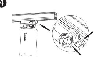
Turn the mechanism 90 degrees to lock the luminarie on the track
