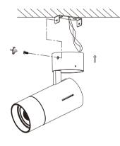
Install the luminarie with the mounting plate by screws
