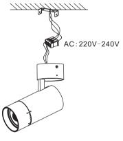
Connect AC cable on the terminal block, Positioned marked with N, L and E
